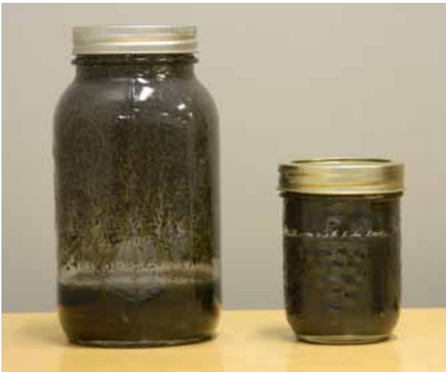
Figure 4.5.2. Stormwater can contain many contaminants, such as tire debris, petroleum, cooking grease, dust and metals. These jars contain stormwater products collected by an oil/grit separator located in a commercial area north of Toronto. If oil/grit separators are not cleaned out, these products would enter lakes and rivers.
